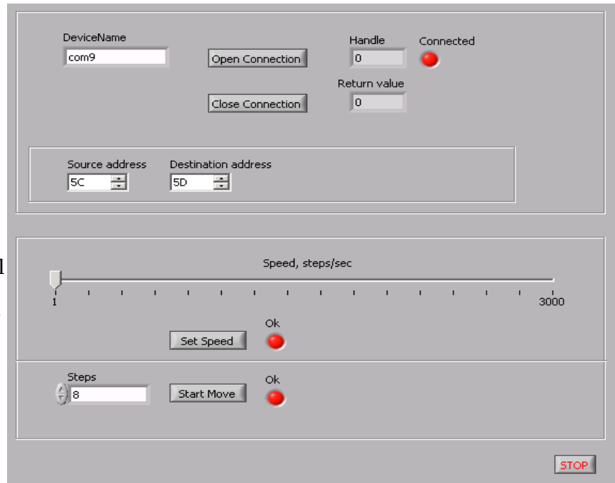
Illustration 1: Simple LabVIEW front panel for controlling motor. The motor is at address 0x5D and the PC at 0x5C, using serial port 9 (com9).
